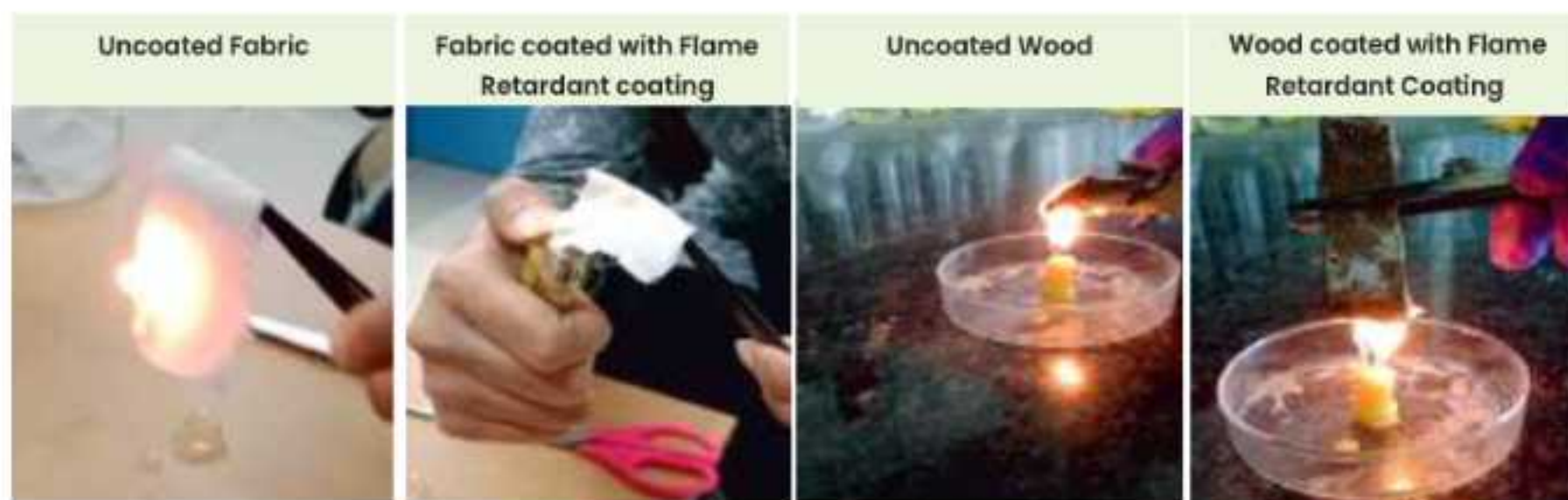
Fig. Uncoated and Flame Retardant Material Coated Wood and Fabric
